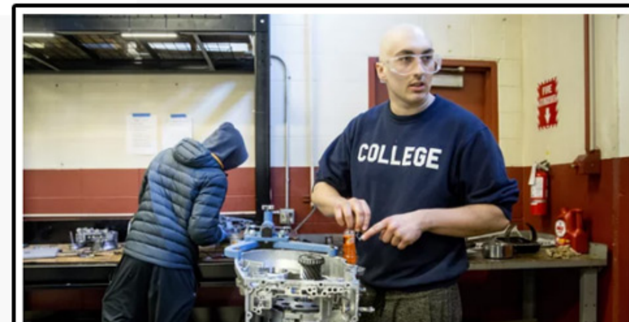
Matthew Dickinson, 21, asks a classmate for help as they rebuild an automatic transmission back in 2018 in a class at the Lake Washington Institute of Technology.
