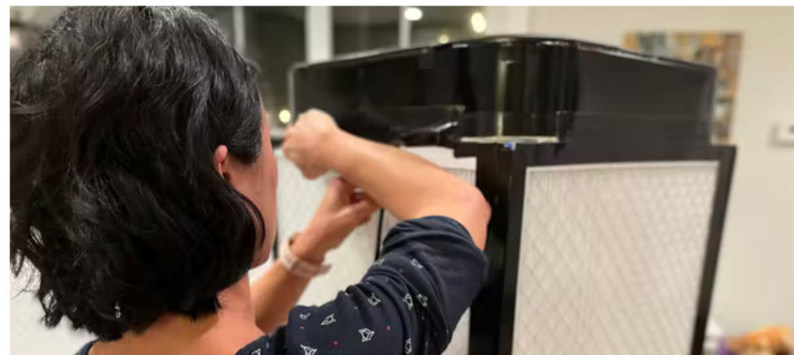
Building a Corsi-Rosenthal box portable air filter comes down to duct-taping together a set of furnace filters and a box fan.
